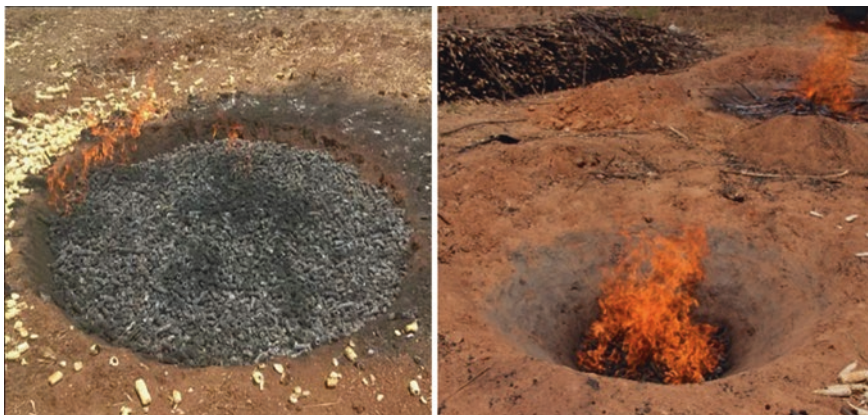
Fig. 1 Pyrolysis in flame curtain kiln in Zambia. (Photo: Left, corncob by A. Obia; right, pigeon pea by G. Cornelissen)
